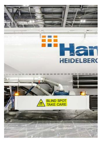
Side under-run protection shall be fitted to both sides of the vehicle (except where this is impractical or proves to be impossible)
